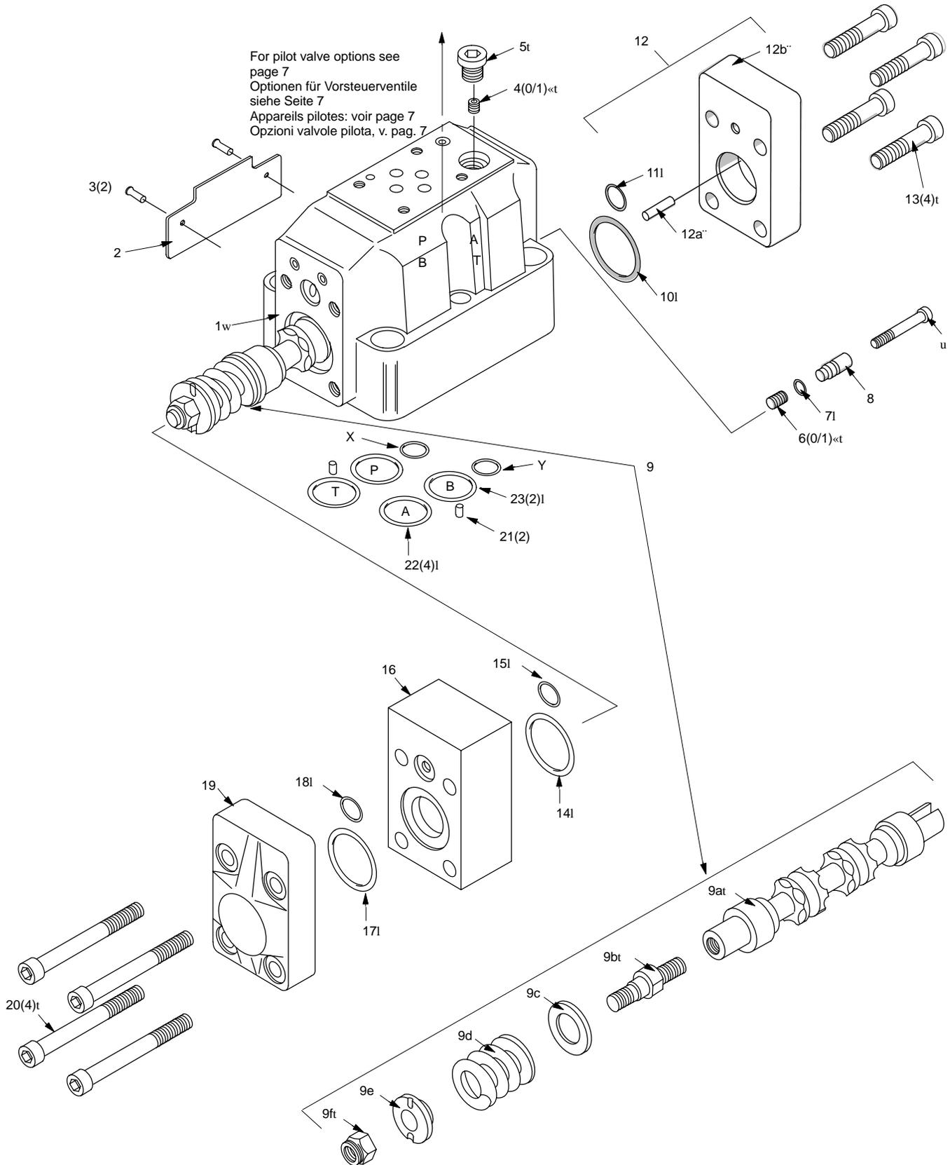
« Factory-fitted plugs, as indicated below, are retained with bonding compound. Removal is not recommended. If installing plugs during field conversion use Loctite 582 compound or similar.
