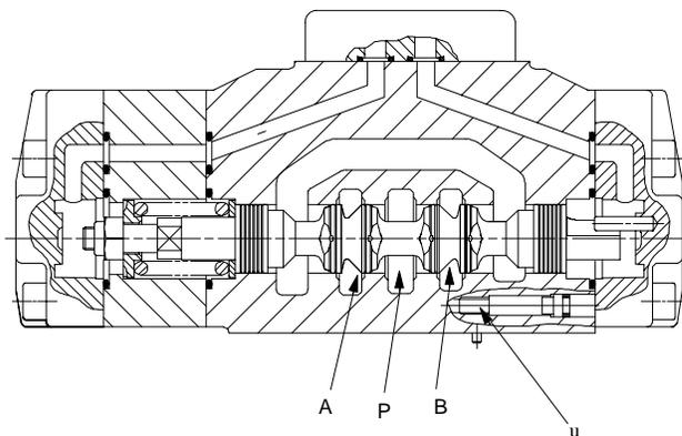
s Plug fitted only in externally drained K(A)DG5V models and in all KDG3V models; see footnote « on page 5.
