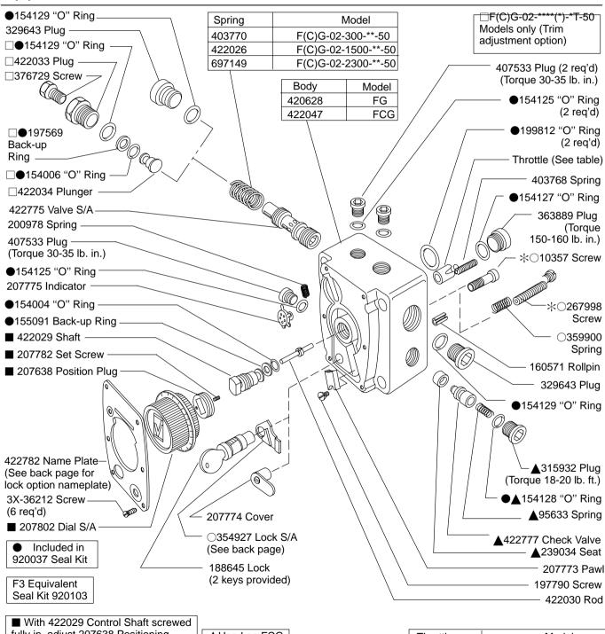
fully in, adjust 207638 Positioning Plug in 297802 dial so that "O" on dial lines up with pointer on nameplate when dial is assembled on shaft. Lock securely with 207782 set screw.
