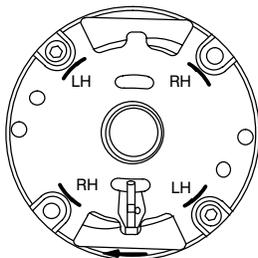
Sharp Edges of Vane Must Lead in
