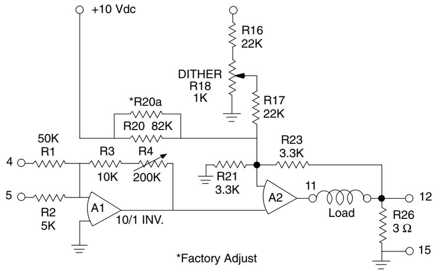
Figure 3. Simplified Schematic Diagram of the EM-A-10
