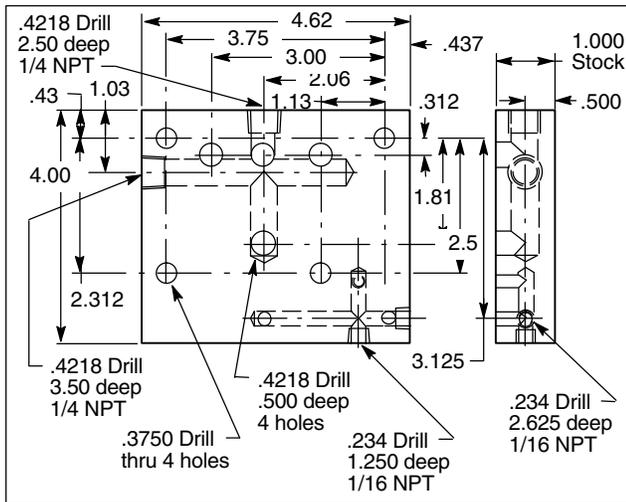
Figure 3. Flushing Plate (938714)
