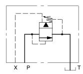
Sequence valve, manually adjusted, CG2V-\*\*\*-1-1\* model▲
