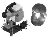
This cutting machine easily handles all one and two braided wire hose through 4" I.D., up to 2" I.D. 4-spiral and up to 1-1/2" I.D. 6 multispial reinforced hose. That makes this machine ideal for cutting most hydraulic and pnuematic hoses as well as a variety of industrial fluid transfer hoses. The T-70 uses a 14" cutting blade for cutting all 1 & 2 wire braid and through 2" 4 spiral hose. The
