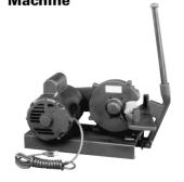
The T-10B hose cutting machine assures quick, clean, right angle cuts, eliminating ragged and frayed cut ends which make hose assembly difficult and are a possible cause of premature hose failure. A powerful 1 H.P. motor and belt-driven blade cut all low, medium and high pressure fabric and wire-braided hose from 3/16" through 1-1/4" I.D. 2 wire hose. Specifically designed for cutting hose, the T-10B is a natural companion to the T-400-1 Coll-O-Crimp and T-300 hose assembly machines.
