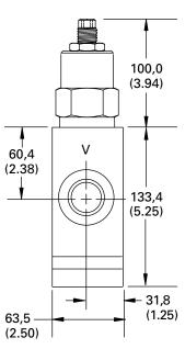
The MCV1-20 is an inline housing type motion control or load holding valve. This valve controls a moving load and prevents loads from running ahead of a pump. It will also lock or hold a load in any position and provides for thermal expansion relief.
