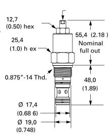
The CBV\*-12 is a 3-ported, externally piloted, screw-in cartridge type counterbalance valve.
