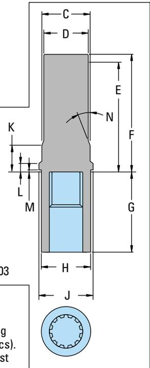
For 2000 Series Bearingless Motor application information contact your Eaton representative (mating coupling blanks available from Eaton Hydraulics). Note: After machining blank, part must be hardened per Eaton specification.
