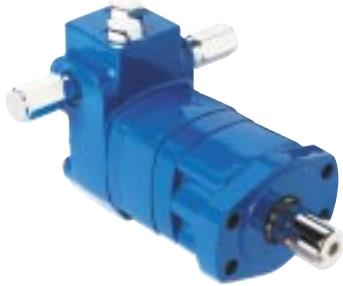
Eaton Char-Lynn®, your proven low speed high torque motor supplier, now offers the Char-Lynn® 2000 Series motor with our proven Eaton Vickers® Screw-in Cartridge Valves integral to the motor. This compact and efficient package offers increased value and cost effectiveness to designing Eaton into your applications. Minimizing the use of hoses, tubing, and fittings will reduce production and assembly time significantly.
