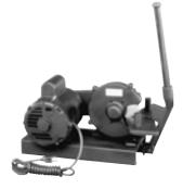
The T-10B hose cutting machine assures quick, clean, right angle cuts, eliminating ragged and frayed cut ends which make hose assembly difficult and are a possible cause of premature hose failure. A powerful 1 H.P. motor and belt-driven blade cut all low, medium and high pressure fabric and wire-braided hose from 3/16" through 1-1/4" I.D. 2 wire hose. Specifically designed for cutting hose, the T-10B is a natural companion to the T-400-1 Coll-O-Crimp and T-300 hose assembly machines.
