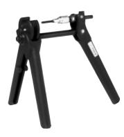
Assembly of Barb-Tite pushon hose ends is made easy with this handy tool. Easy and fast operation assures dependable, leak proof assemblies. Simply clamp hose in jaws, place hose end on push rod and pull the handle. Engineered for a lifetime of rugged service. Weight: 1 lb. Capacity: 1/4" to 1/2" I.D. hose only.
