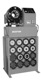
The T-605VS is designed for high-speed production crimping of hydraulic and fluid transfer hose assemblies. Equipped with Boston "bump-and-skirt" dies, the T-605VS produces OEM-quality crimps on Eaton 'U', '430U' and 'E' series hose ends. Optional flat-crimp dies allow crimping of other Boston hose ends and Boston Wolf Couplings.
