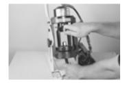
5. Holding the uncrimped hose assembly in place throughout the crimping operation, pull the pusher positioning handle as far forward as it will go. The pusher will now be in the proper position for crimping. Hold down on activation button and start crimping.
