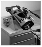
repair of all your hose needs and designed to be used in remote or portable stations, the ProCrimp 1380P will handle through -20 SAE100R12 hose and fittings. All die cages, crimp diameters and approved hose and fitting combinations are identical to Eaton's popular FT1380 crimper. Crimp diameters are controlled using a micrometer and specially designed hydraulic circuit that allows
