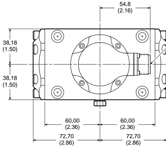
Electrical connector mates with MS-3106-14S-2S (4 pin). Plus signal to A or C causes flow out of port B.
