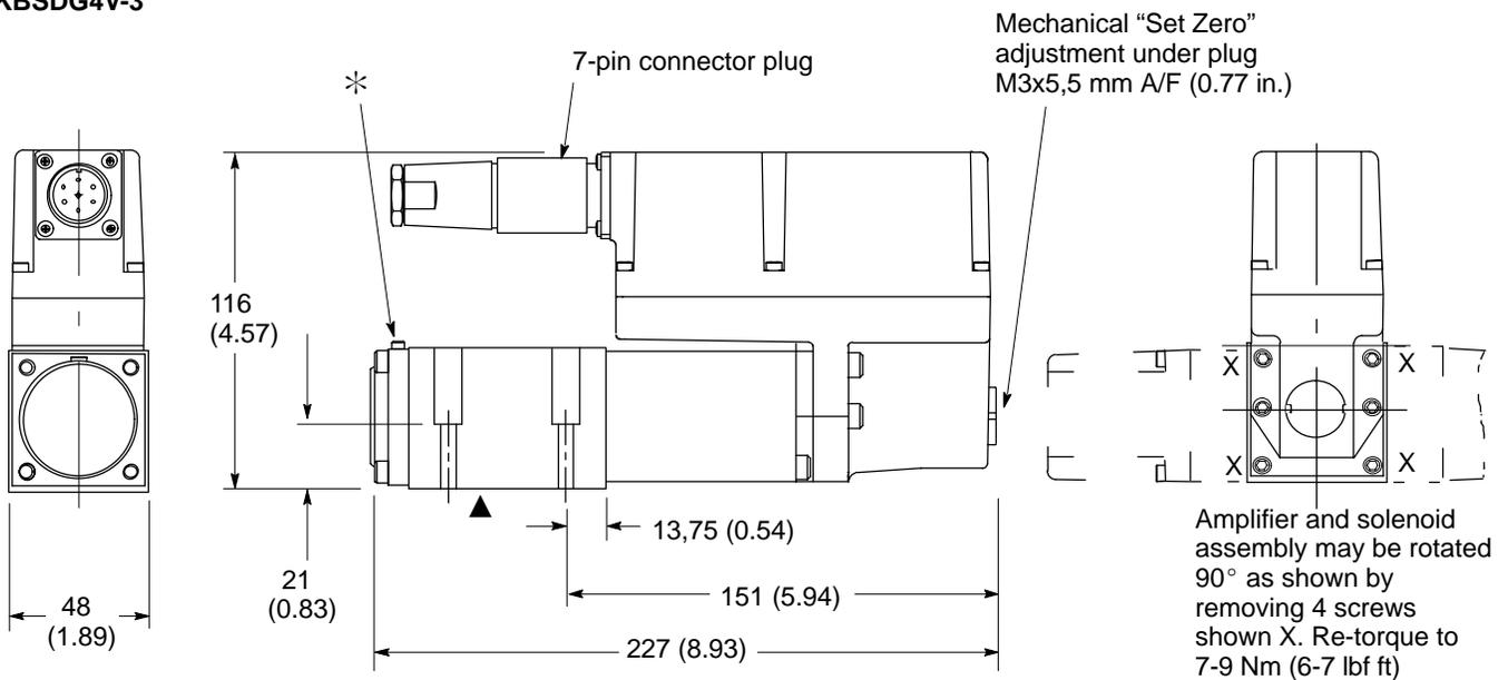
▲ Mounting surface seals supplied. For mounting surface dimensions and subplate options see page 9.
