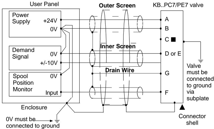
■ Spool position monitor voltage (pin F) will be referenced to the KB valve local ground. A "local ground" (pin C) is provided on PC7/PE7 versions for optional use by differential input customer supplied electronics.
