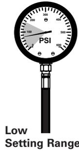
F. Slowly rotate the neutral adjustment screw clockwise until charge pressure drops to its low setting. Mark the neutral adjustment screw location.
